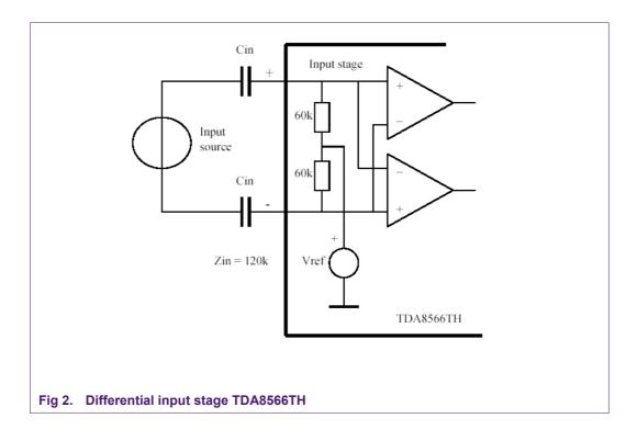
Furthermore it is recommended to use input capacitors with a low DC leakage (film capacitors), since any DC leakage at the inputs will result in a DC offset at the outputs. Electrolytic capacitors usually have a relatively high DC leakage and should therefore not be used.
