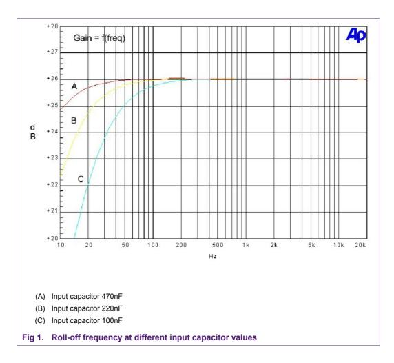
The low frequency roll-off point can easily be calculated :
